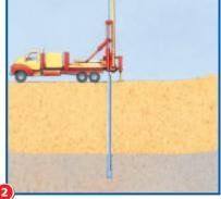
When the drill hole reaches below the water table, lower a pipe into it.
